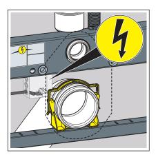
Lay the power supply for an electric flush plate up to the cavity wall socket.
