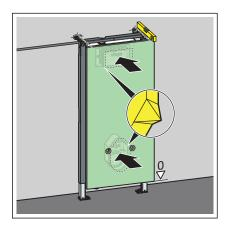
Corn the gypsum cardboard cladding panel at the revision shaft and at the site protection by applying gentle pressure.
