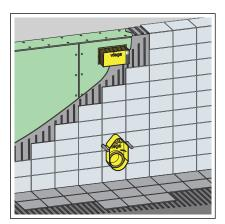
■ Clad the element with suitable gypsum cardboard cladding panels.
