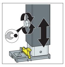
Loosen the feet of the element using a fork spanner.
