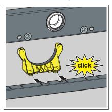
■ Insert the mounting bracket for the drain elbow.
