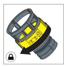
Lock the flushing throttle.
