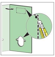
Cut out the recesses for the site protection, the revision shaft and the threaded rods.
