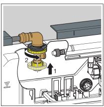
Use the lock nut to screw the corner valve and the cistern to each other.
