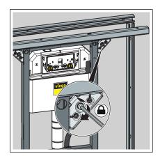
Fix the element with the Prevista Dry Plus rail connectors.
