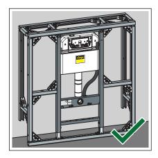
$\hfill \hfill \square$  The WC element is fixed in the Prevista Dry Plus pre-wall construction.
