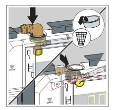
**INFO!** For the concealed cistern 3H, the corner valve can be attached from the top or rear.
