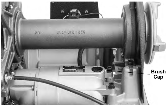
Figure 34 – Removing Motor Cover/Changing Brushes
