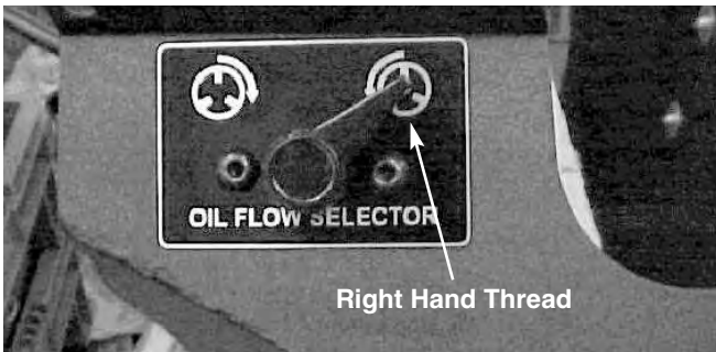
Figure 24 – LH or RH Oil Flow Selector
