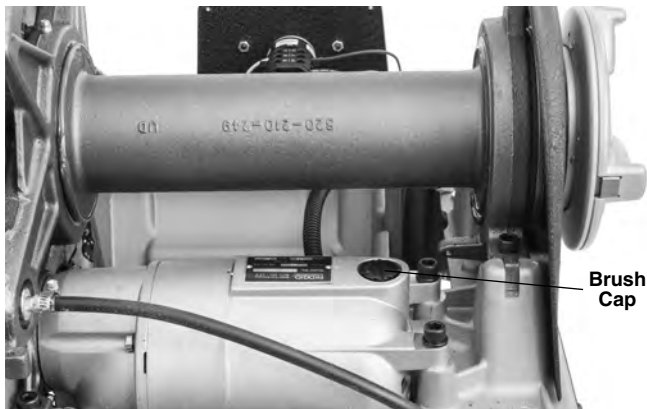
Figure 34 – Removing Motor Cover/Changing Brushes
