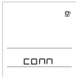
During initial operation, room unit address is set automatically. If one room unit is connected, it acquires address 1. If an additional room unit is connected, it acquires address 2. If two room units are connected simultaneously, address has to be confirmed or set on one of them, and the other room unit automatically acquires the remaining address.
