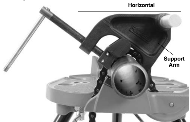
Figure 11A – Positioning the Support Arm
