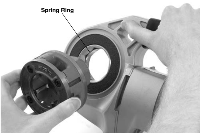
Figure 9 – Installing Die Heads into 600-I Power Drive
