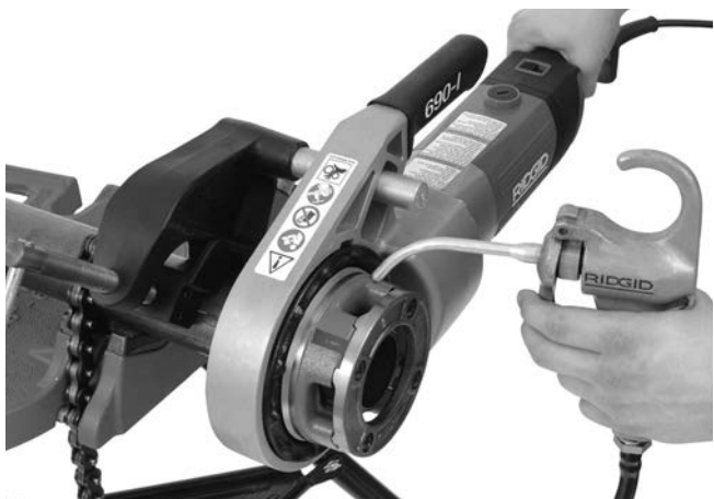
Figure 14 – Filetage du tuyau
