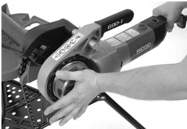
Figure 13 – Entamer le filetage
