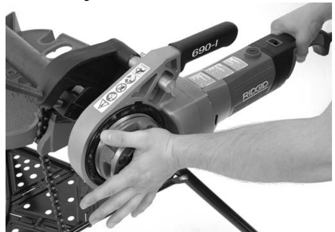
Figure 13 – Starting the Thread
