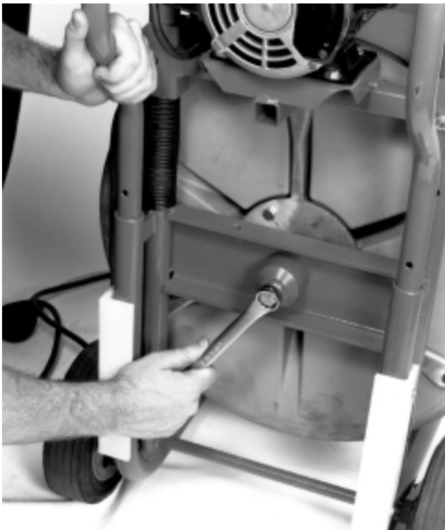
Figure 9 – Remove Bolt Which Fastens Drum Assembly to Machine Frame
