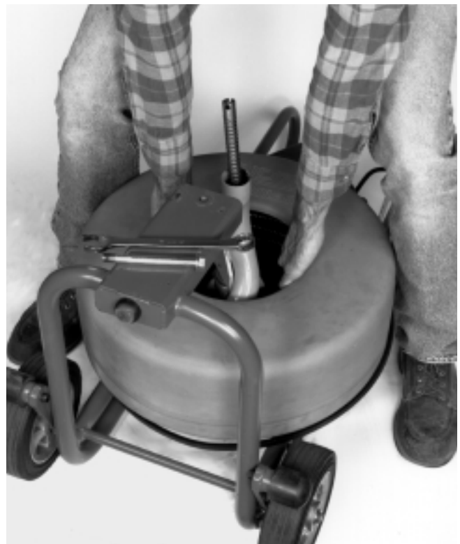
Figure 10 – Lift Drum from Mounting Position
