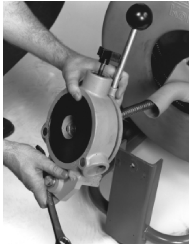
Figures 7a and 7b – Use \frac{3}{4} " Wrench to Remove Autofeed Assembly
