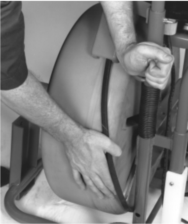
Figure 8 – Release Belt Tension
