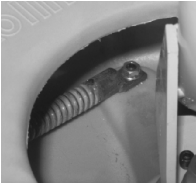
Figure 11 – Removing Pigtail Anchoring Bolt
