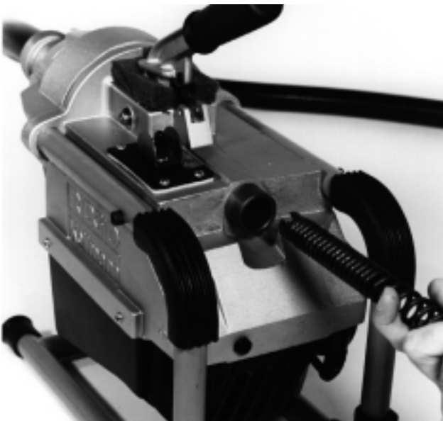
Figure 5 – Inserting Cable Into Front Of Machine
