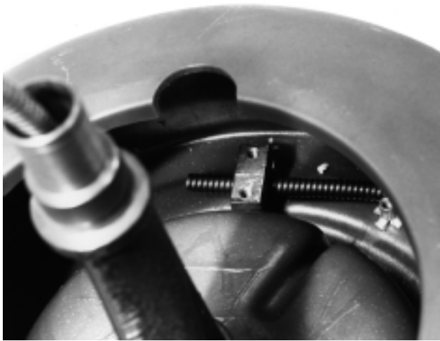
Figure 16 – Position New Cable Under Bracket
