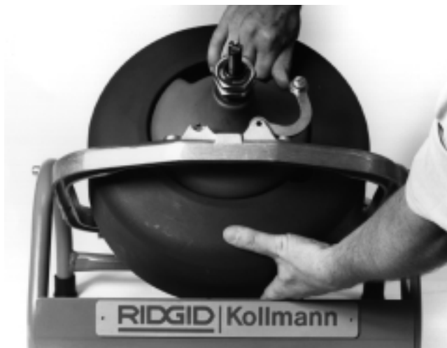
Figure 2 – Aligning Drum and Gearbox Bore
