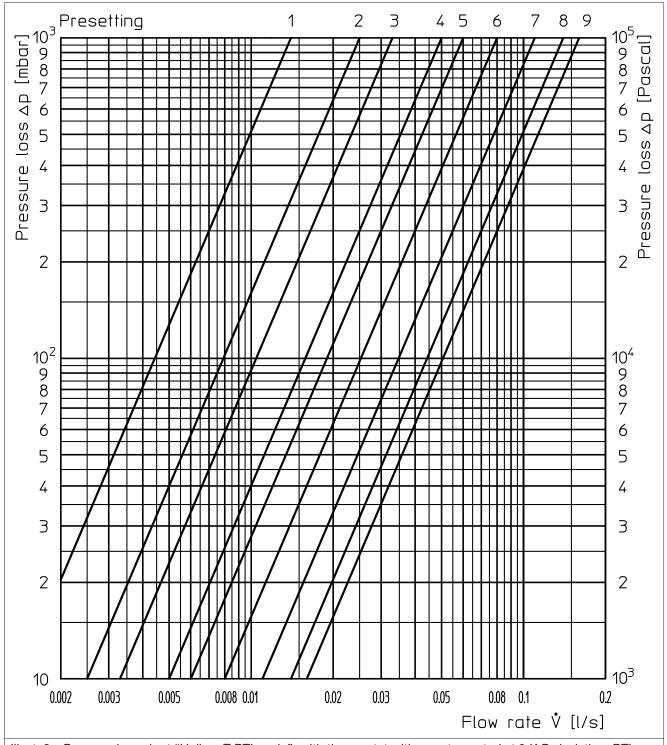
Illust. 3: Pressure loss chart "Unibox T-RTL vario", with thermostat with remote control at 2 K P-deviation, RTL fully open
