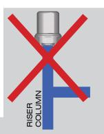
In locating the water hammer correct position in a system, it is important to avoid creating areas where stagnant water may remain, i.e. situations where bacterial colonies can proliferate. For instance, installations at the top of a riser column can create areas with still water ("dead zones"), even though the water hammer arrester will function properly. Consequently, this kind of installation must be avoided.
