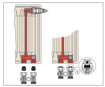
Caleffi panel radiator valves are designed to be installed on panel radiators featuring connections both on the bottom and an externally invisible inner pipe, which feeds the flowing medium to the upper valve.
