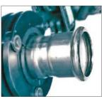
Turn the press collar into the appropriate position for applying the pressing tool. Open the pressing tool by pushing down the lever of the intermediate adapter and apply it on the press collar in such a way that the claws of the intermediate adapter grip around the bolts of the press collar. Then check whether the outer edge of the fitting corresponds with the marking.
