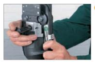
Select intermediate adapter to suit the dimension. On electronic press machines for dimensions from 40 mm to 63 mm and for conventional press machines, insert intermediate jaw ZB 203 (SANHA catalogue no. 6930) in the press machine and close the retaining bolt.
