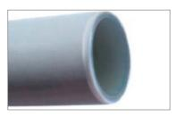
3 Check that the end of the pipe is clean and properly deburred (visible by a circumferential 15° chamfer).
