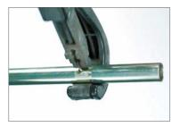
1 Cut pipes to length at a right angle using either a pipe roll cutter suited to the respective material or a fine-toothed metal saw.
