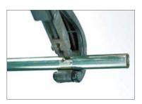
1 Cut pipes to length at a right angle using either a pipe roll cutter suited to the respective material or a fine-toothed metal saw.
