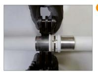
Select suitable press collar. Ensure that the marking lines on the sliding segments and the press collar collets form one line. If this is not the case, loosen the sliding segments.
