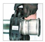
The press collar can only be removed from the press joint if both intermediate jaws (ZB 321 and ZB 322) were used.
