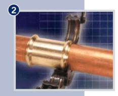
Select the appropriate collar and open by depressing the spring loaded pin. Pull apart and position over the fitting.
