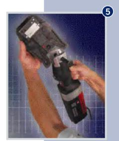
Depress the button on the press tool and begin the pressing operation.
