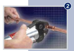
Depress the trigger/button to begin the compression cycle of the tool. This is complete when the mouth of the fitting is fully enclosed by the jaws. Now release the jaws from around the fitting. (For further information refer to tool manufacturer's instructions.)
