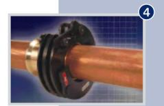
Take the appropriate adaptor and attach to the press tool, then close the breach bolt. To attach the collar, depress the jaw levers and attach the claws as far as you can into the grooves of the collar. Unless the adaptor is correctly connected to the press collar pressing will not be possible.
