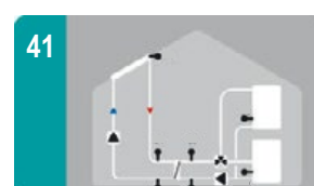
Solar with 2 storages, heat exchanger and valve for large systems
