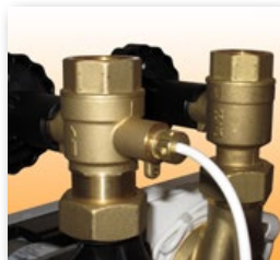
Supply isolating valve with built-in pit for the insertion and the lead sealing of the hot water sensor.
