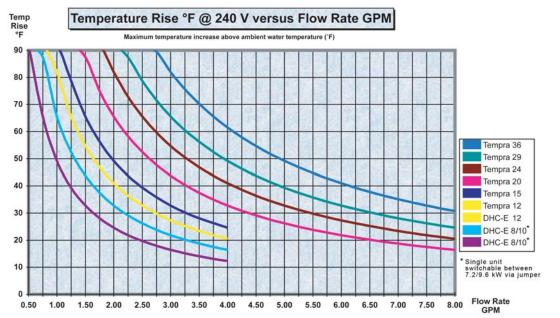
$<sup>^{\</sup>star}$  Suitable for supply with up to 131°F / 55°C  $^{\star}$  Tankless water heaters are considered a non-continuous load
